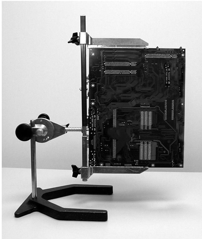
Figure 1-8: Setting up a Rambus mother board
